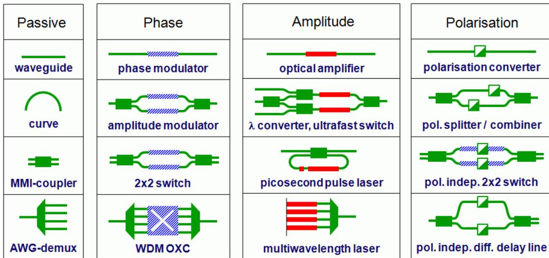
*Figure 3 Example of the functionalities that can be realised in a generic integration technology that supports four basic building blocks: Passive Waveguide Devices (PWD), (Optical) Phase Modulators (PHM), Semiconductor Optical Amplifiers (SOA) and Polarisation Convertors.*
