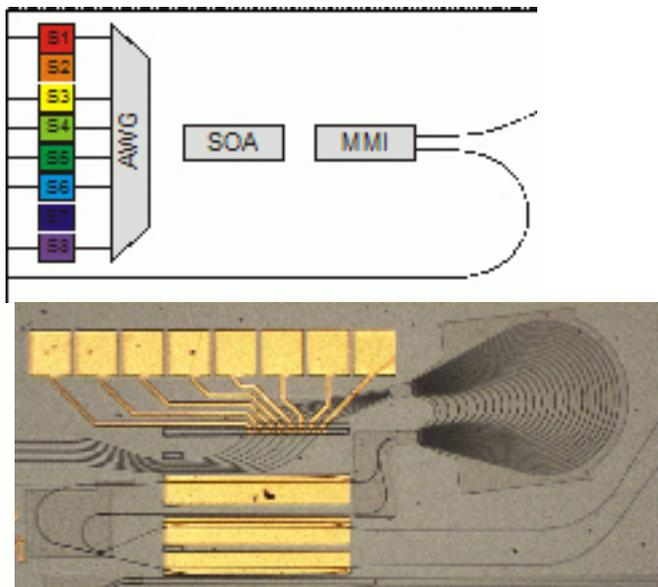
*Figure 4 Circuit scheme and microscope photograph of a fast discretely tuneable laser with 100GHz channel spacing which has recently been realised in the COBRA InP-based generic integration process. Chip dimensions are  $1.5 \times 3.5\text{mm}^2$  [4].*
